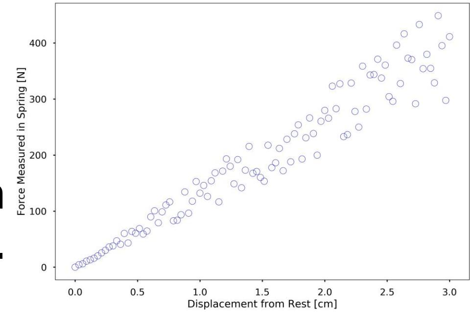
How to estimate model parameters (e.g., stiffness) given a set of data?
