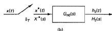
Figure 3-4 (a) A real sampler and zero-order hold; (b) mathematical model that consists of an impulse sampler and transfer function G_{H0}(s)
